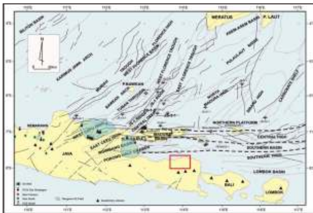
Figure 3. Elements of the East Java Basin regional tectonics and hydrocarbon occurrences information. The research area is shown in blocks.
